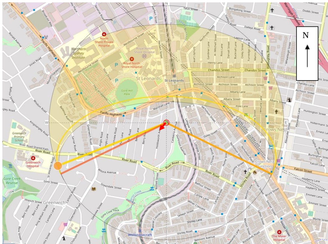
Figure 11: Representation of incident and reflection of solar rays from the south-west façade onto Holdsworth Avenue.
